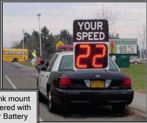
Trunk mount powered with Car Battery
